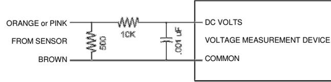
Best accuracy and noise immunity is obtained by connecting a 500Ω resistor to the current return wire at the measurement point. The default configuration is for calibrated output, with the zero point at zero distance, and the span at full scale.
