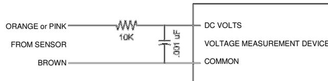
Best accuracy and noise immunity is obtained by connecting a 10KΩ resistor to the voltage return wire at the measurement point. The default configuration is for calibrated output, with the zero point at zero distance, and the span at full scale.
