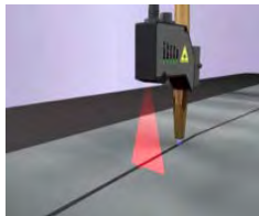
Weld Seam Tracking
