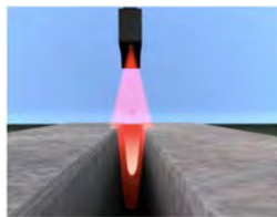
Measurement of Gap and Flushness
