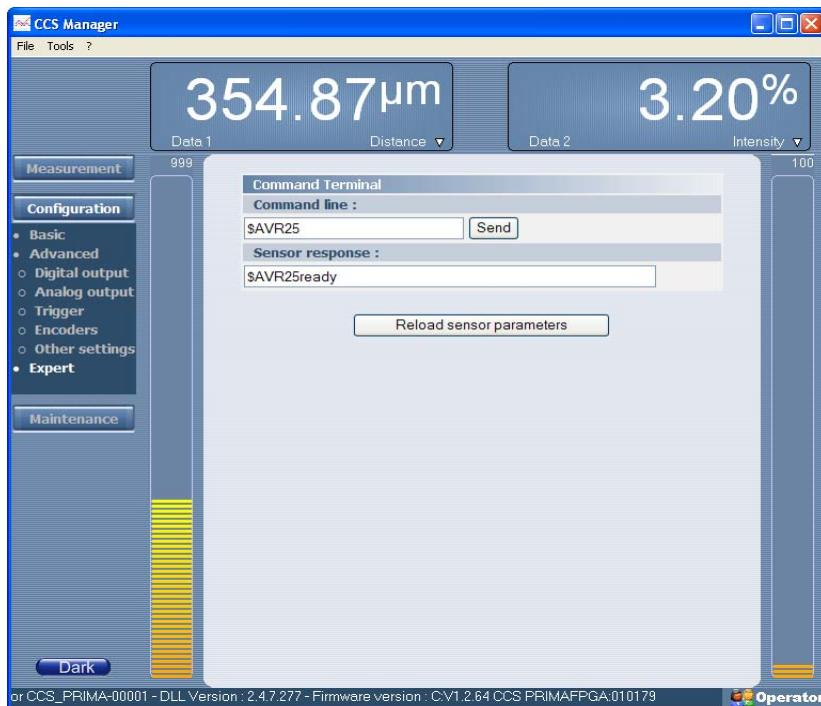
Figure 10 Built-in terminal program in CCS Manager
