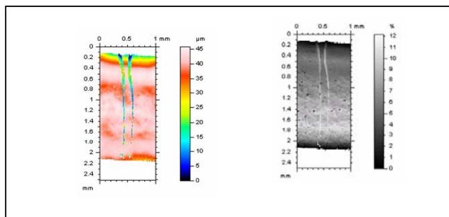
Figure 8 "Distance" Image (left) and "Intensity" image (right) of a scratch on the neck of a glass bottle.
