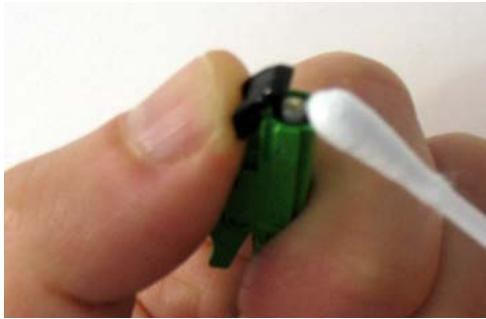
Raise the black protecting cap over the fiber optics plug, and clean the fiber optics tip carefully. Use absorbent cotton, or a paper towel, soaked with alcohol (e.g. Ethanol or Methanol). Perform circular movement so as to push the dust grains away from the fiber tip.
