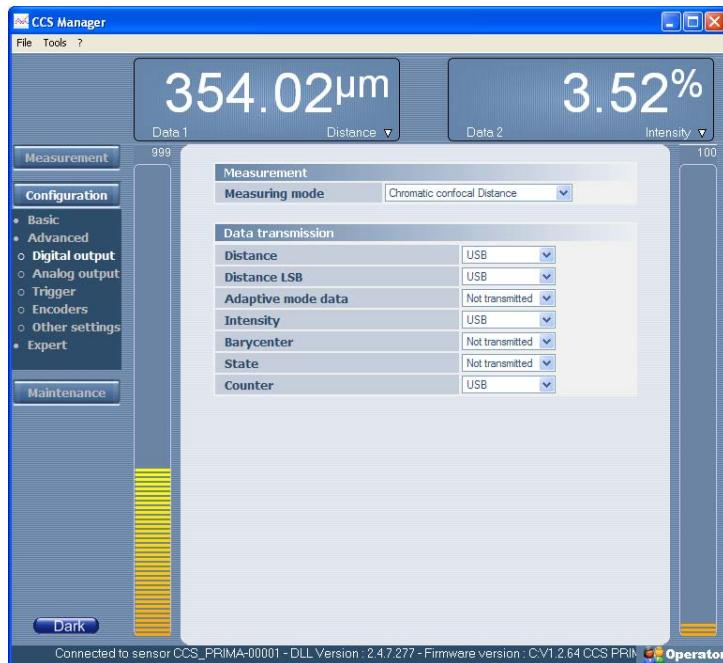
First, observe the list of available data items in the "Distance" measuring mode. In this mode you can measure the Distance and the Intensity of the reflected signal.
