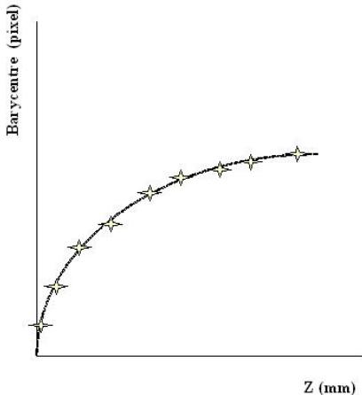
The relation between the position of the spectral peak ("barycenter" in pixels) and the axial position of the object ("distance" in  $\mu\text{m}$ ) is called "calibration lookup table" (LUT).
