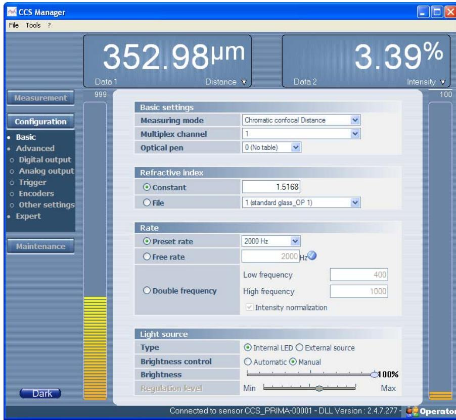
Set the measuring mode to "Distance" and then select a Preset Rate of 100 Hz.
