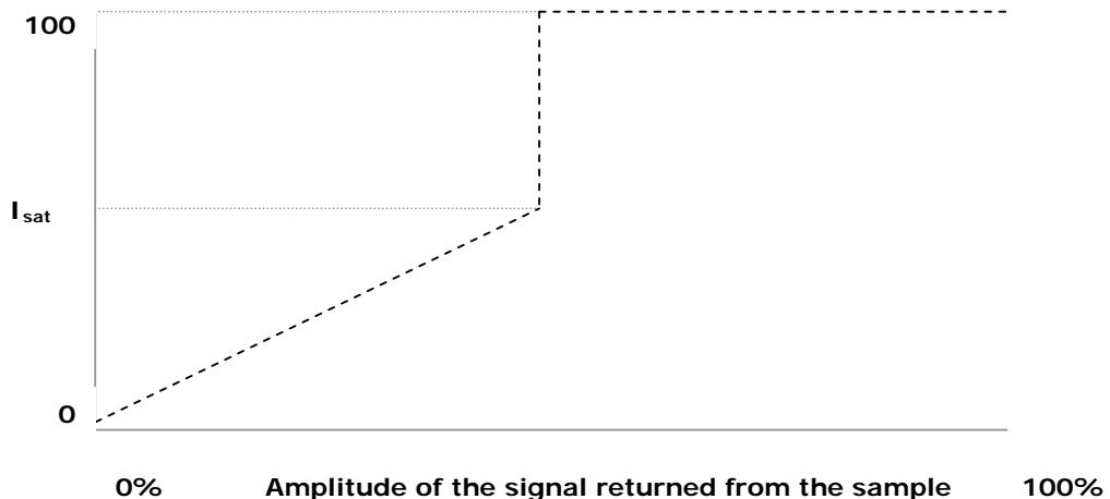
The value of  $I_{sat}$  depends on the detection wavelength  $\lambda_o$ , and may vary slowly within the measurement range of the sensor. For some wavelengths  $I_{sat}$  equals 99%. For others it is lower.
