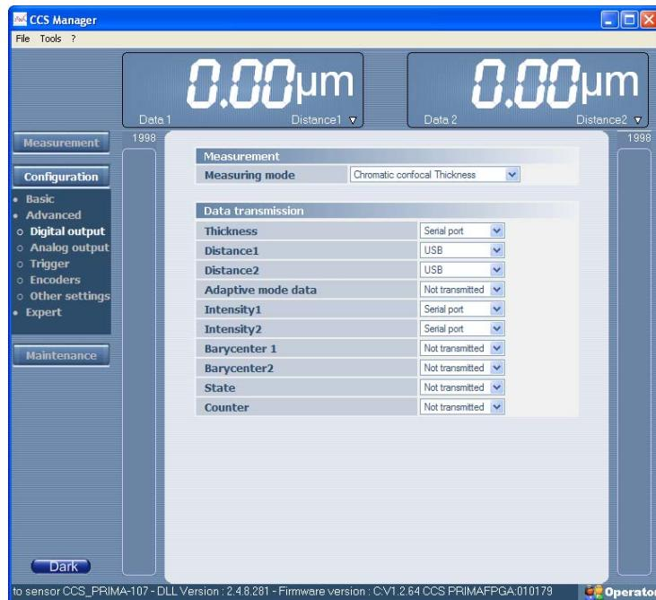
In the screen copy above, the thickness and the intensities are directed to the RS232, while the 2 distances are directed to USB. In this way one can connect the sensor to two applications simultaneously (e.g. HyperTerminal on the serial port and CCS manager on the USB port).
