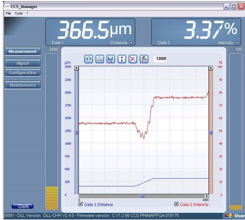
In the "Data 1 frame" on the top of the Main Window the list shows the transmitted data items (Distance, Intensity, and Counter). Select data1 as "Distance"; In the "Data 2" frame Select "Intensity".
