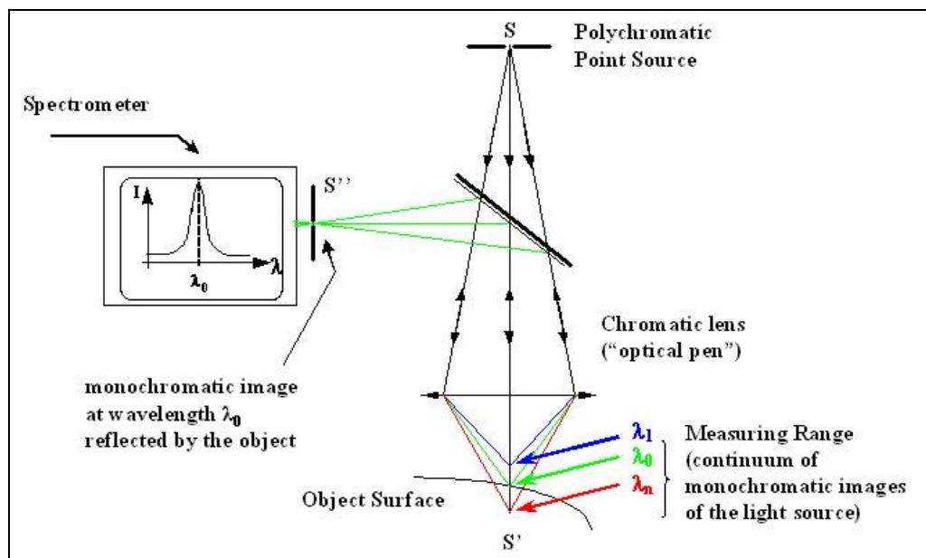
Figure 5 Description of Chromatic Confocal Imaging
