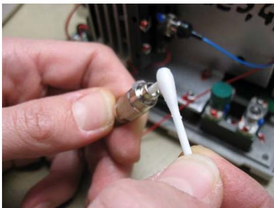
Replace the optical fiber on the feed - through connector.
