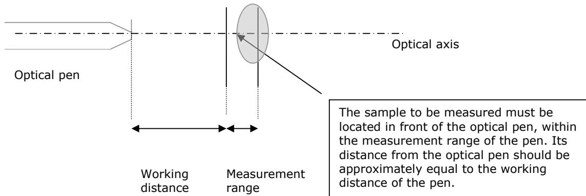
As soon as the sample is located inside the measuring range of the optical pen, the "Measurement" LED indicator on the sensor front panel lights on. Once the sample is
