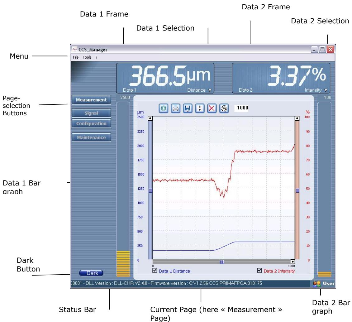
Note: the "Signal" page-selection button does not appear in the "Operator" level.
