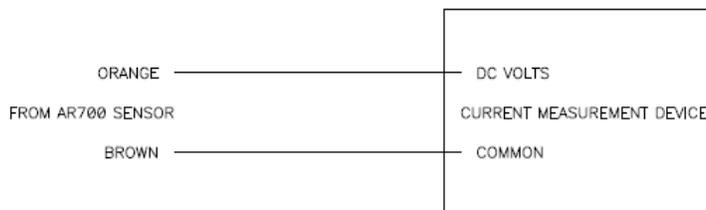
The best conversion to voltage is obtained by connecting a 500-ohm load resistor (1/4 Watt minimum) between the orange and brown wires at the measurement point. This gives a 2 volt to 10 volt output range.
