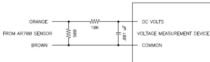
The sensor may be connected directly to a meter or a filter may be inserted to reduce noise. The filter shown will pass the signal at full speed (nearly 10000 samples per second). To filter better at slower speeds, use a 0.01 uF capacitor (1000 samples per second) or a 0.1 uF capacitor (100 samples per second).
