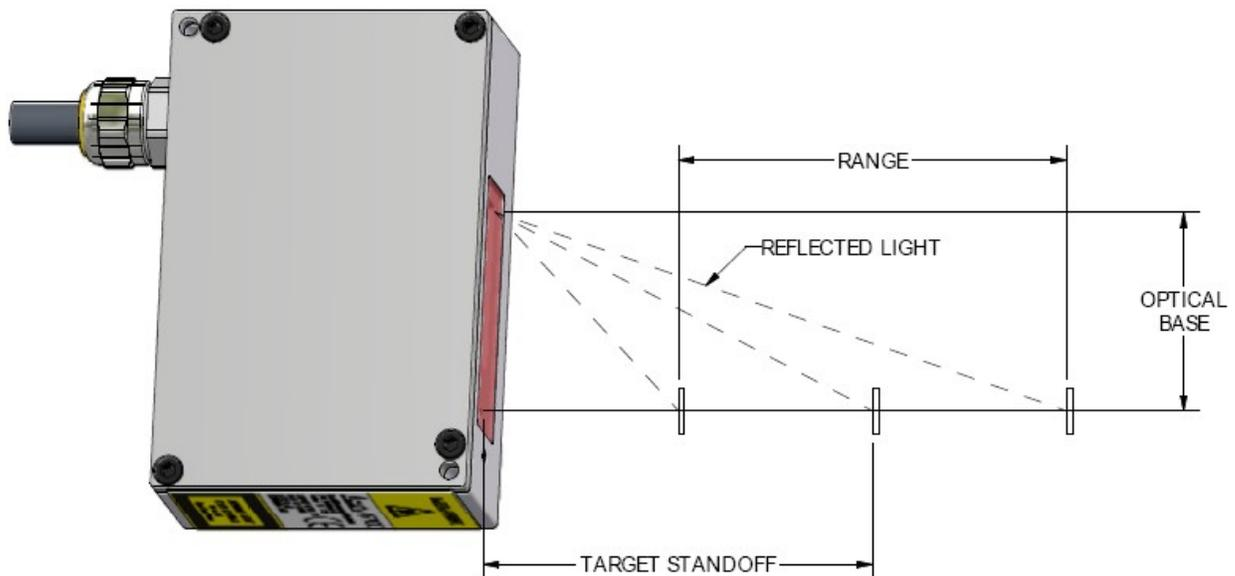
Laser light is emitted from the laser aperture, which is close to the “Laser Aperture” placard as shown. The laser beam then strikes the target at a position along its range. Some of the laser light reflected from the target is collected by the camera lens.
