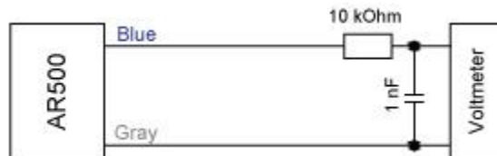
Figure 4 Wiring Diagram for Voltage output
