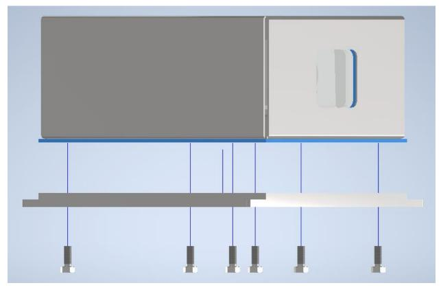
Do not remove any fasteners around the viewport unless to replace a damaged window. These will be 7mm hex nuts on the inside of the enclosure.
