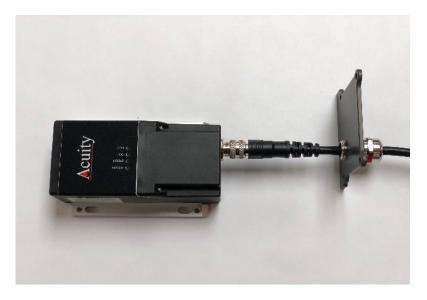
First, insert the cables into the cable glad of the jacket. Then connect the cable to the sensor before you assemble the laser sensor into the aircooling jacket.
