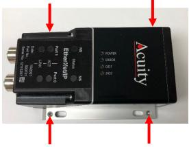
Remove the four hexagonal socket set screws. You need these tapped holes to mount the sensor into the jacket.
