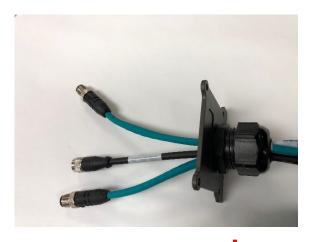
Insert the cables into the cable gland of the rear cover. Then push the rubber seal into the cable gland.
