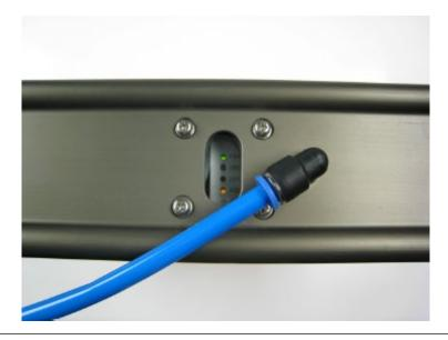
The user can see the sensor's operating status through the clear glasses on the housing top without pulling the laser sensor out. This makes it convenient to do maintenance or monitoring device on site.
