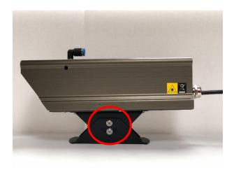
The tilting can be adjusted with the four screws on the two sides of the air jacket.
