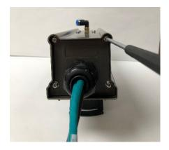
Fasten the cable gland after adjusting an appropriate cable length to be inserted.
