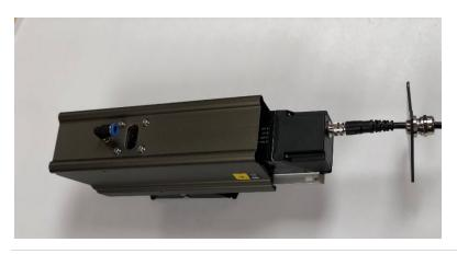
Slide the wired sensor into the air jacket.
