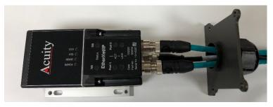
Connect the power and ethernet cables to the sensor
