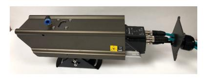
Slide the wired sensor into the air-cooling jacket.
