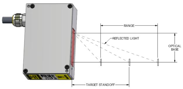
Laser light is emitted from the laser aperture, which is close to the "Laser Aperture" placard as shown. The laser beam then strikes the target at a position along its range. Some of the laser light reflected from the target is collected by the camera lens.
