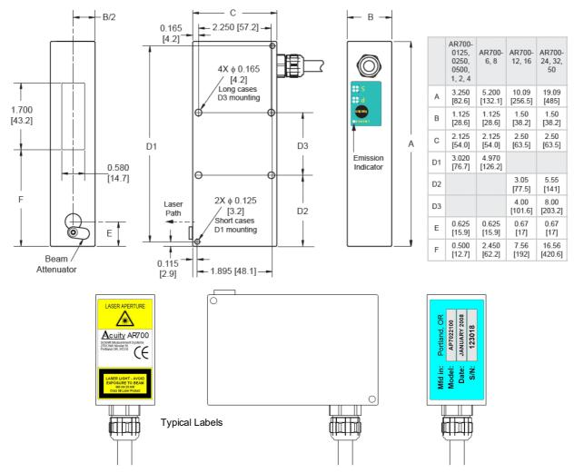
The Beam Attenuator is supplied for Class 3B sensor models. Rotate the beam attenuator to block the laser aperture as required in your system. The sensor will not operate correctly with the beam blocked.
