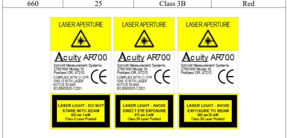
The laser safety classification reflects worst case situations. The laser is considered to be continuous, not pulsed. When the laser pulses in normal operation, the level of laser light does not increase.
