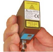
**Standoff:** Offset distance from the face of the sensor to the middle of the span. Accuracy is greatest at the standoff distance and the laser spot size is smallest at this focal point. AR700 standoff location tolerance is +/-0.25mm.
