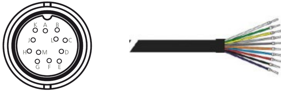
Figure 10 AR3000 multipurpose cable with 12 conductors plus shield and corresponding pin arrangements
