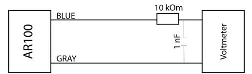
Figure 2 Wiring Diagram for Voltage output
