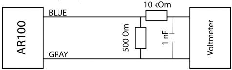
Figure 1 Wiring Diagram for Current Loop output
