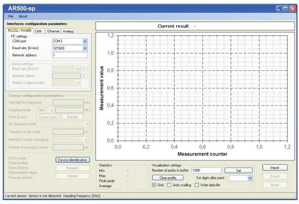
In the RS232/RS485 tab, select the COM-port Where: the sensor is connected. If using a USB to RS232 adapter, look at your computer's hardware profile to determine the assigned COM port. Select the Baud rate noting that the factory default is set to 9600 baud. Select the sensor network address, if necessary. Press the **Device identification** button.
