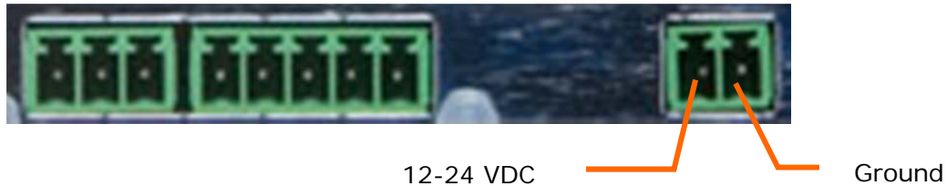
Figure 1. Terminal blocks on rear of TPD
