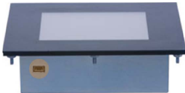
Figure 8 Location of USB port to connect to a PC computer
