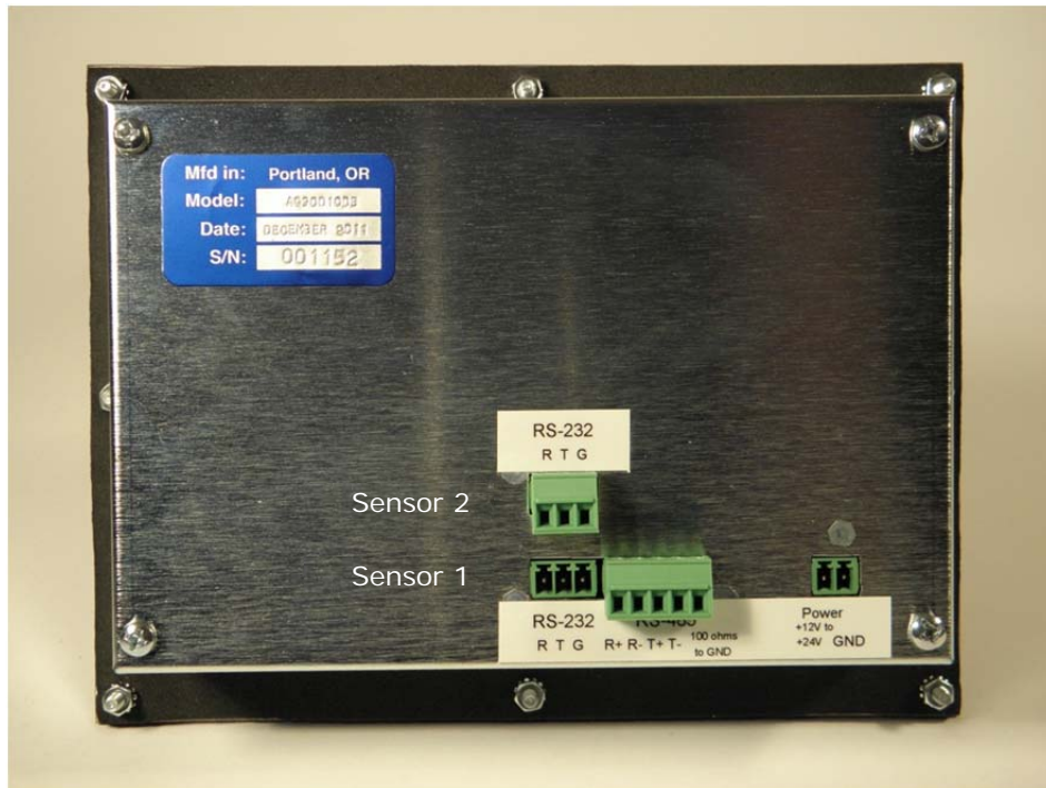
Figure 4. Rear of TPD showing connection blocks for Sensor 1 and Sensor 2
